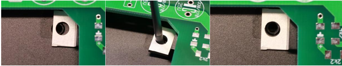
Fig. 3 a, b + c: Positioning of the transistors on the chassis using a screwdriver such as a TORX T8.
