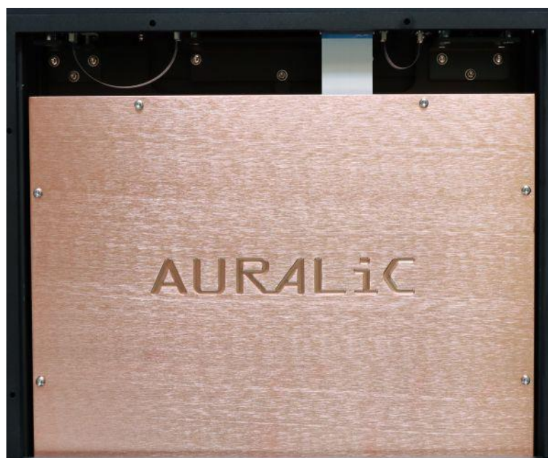
Figure 2: Copper-shielding inside. Loosen 6 screws TORX T10 and put the lid aside.
